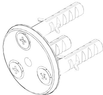
6. Install Grab Rail: Line up the grab rail with the wall plate and screw the wall nut.
