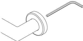
2. Use the grab rail as a template and mark up your holes with a pencil. If you are mounting onto tiles, keep the holes away from the edges of the tiles. If you are mounting onto Masonry use the wall plugs provided.
