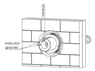
13. When the valve is rotated fully anticlockwise, the top slot should face vertically. [If perfect alignment is not possible, remove it and engage it in the next available spline in the clockwise direction. Then grip this *gently* with vice-grips (or the tool provided) and rotate it anti-clockwise (it should turn the valve cartridge) until it is perfectly square.]
